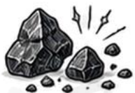
Brittle (e.g., coal or sulphur breaks)
